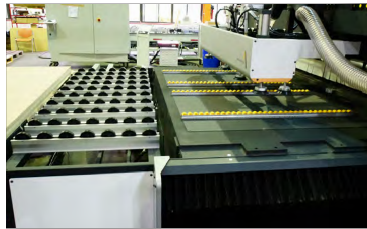
Roller System for loading Panels
