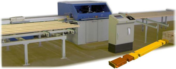
Fully automated Loghouse milling machine Blockhausfräse BL100A for economic production of components used in modern log cabin construction.
