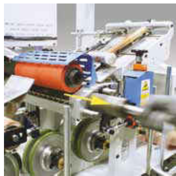
Fast extraction of the applicator roller(RP30).
