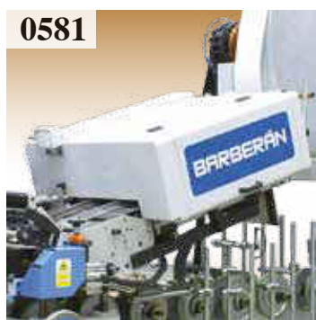
0581 Device for cutting the veneer or CPL from the roll before gluing.
