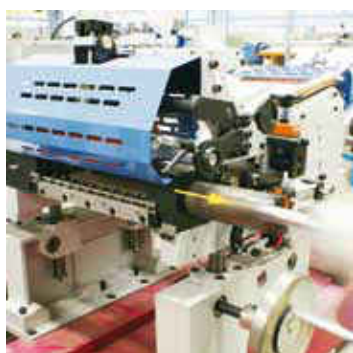
Applicator roller with fast disassembling. (PL)
