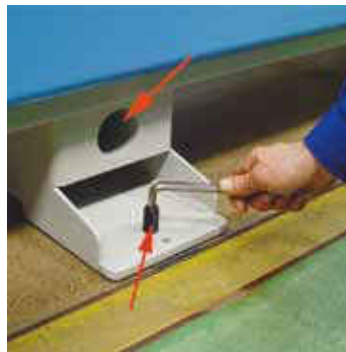
Housing to enable the loading and transport of the machine. Levelling system of the bedframe with key.
