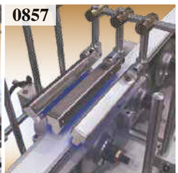
0857 3 Blue light lamps for the visual control of the "PRIMER" applied on the profile.
