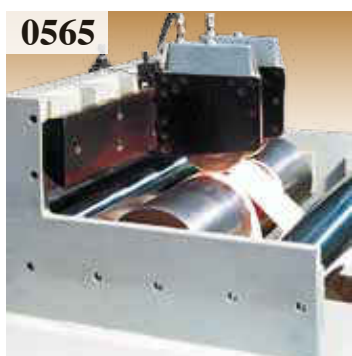
0565 Device to cut the foil before wrapping.
