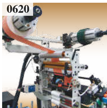
0620 Double unwinding station with manual splicing device with air shafts.
