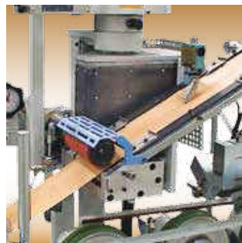
Roller system hot melt application head. (RP-15)
