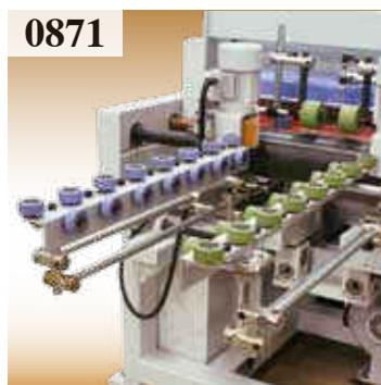
0871 Guides with rubberised wheels for PVC profiles.
