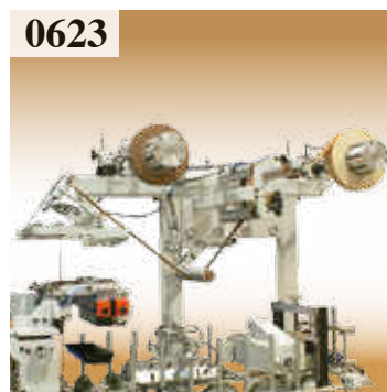
0623 Automatic paper or PVC foil splicing device.
