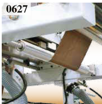
0627 Automatic tensioning system of the two spools for a constant tension.
