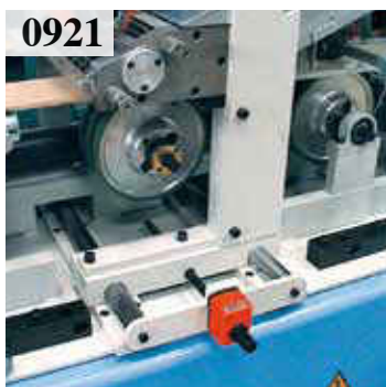
0921 Manual shifting of the hotmelt nozzle to change the wrapping centre.
