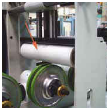
Adjustable first moulding roller. (PUR)
