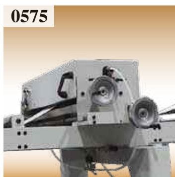
0575 Paper and PVC foil cutting device.
