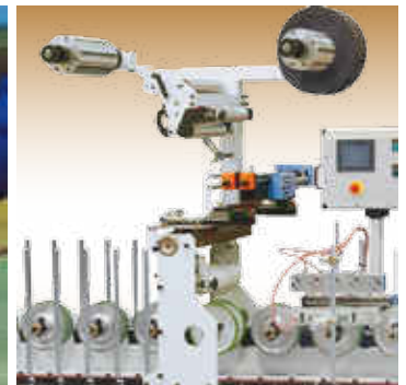
PUR hotmelt glue head, slot nozzle type. (PUR)
