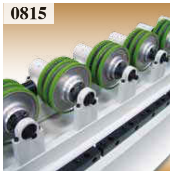
0815 Wheel shaft, supported at both ends, for flat panel wrapping.
