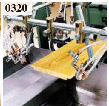
0320 3 guns + stainless pump for PVAc glue application.
