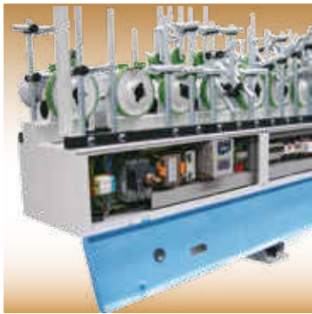
Built-in electrical cabinet.
