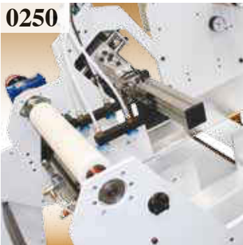
0250 Automatic feeder of HPL or wood veneer strips by means of a suction pad line.
