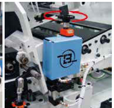
Hot melt dosing adjustment. (RP & PL)
