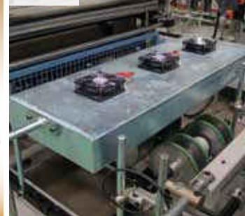
IR screen for panel or profile pre-heating (RP & PL)
