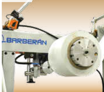
Standard spool continuous automatic brake regulation.
