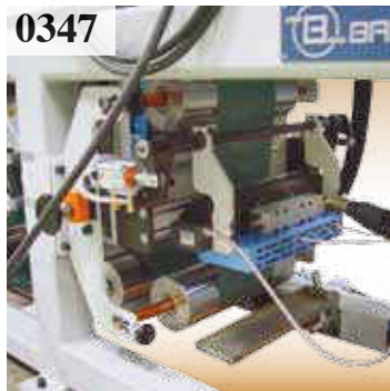
0347 Bottom support with uncoiling station and slot nozzle head.
