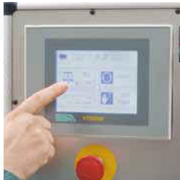
Glue grammage regulation system through PLC. (PUR)
