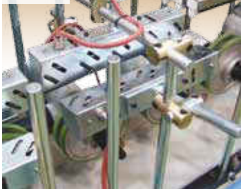
IR screen for profile preheating and laminate softening (1000W).
