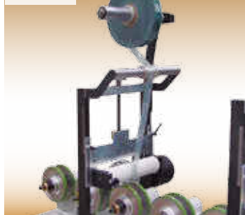
Standard spool continuous automatic brake regulation.
