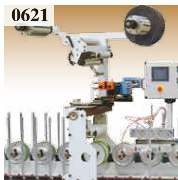
0621 Second roll with half-automatic splicing device. (PUR)
