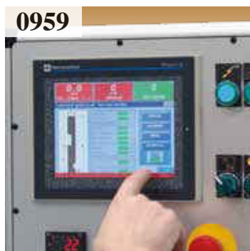
0959 CNC program for the automatic drawer side wrapping tool positioning.
