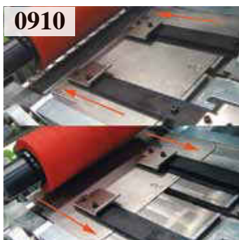
0910 Foil blocking system, gluing roller automatic hiding.
