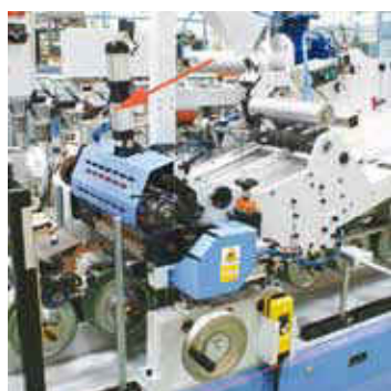
Counter-pressure roller pneumatically driven. (PL)
