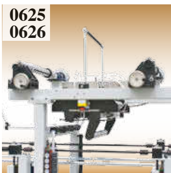
0625/0626 Automatic paper or PVC foil splicing at high speeds.
