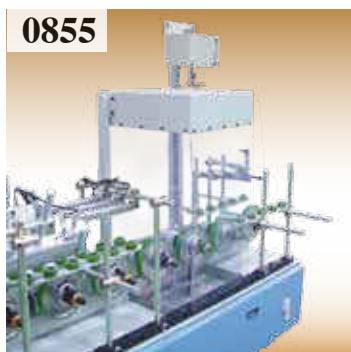
0855 PRIMER station with tank and application pads.
