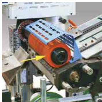
Counter-pressure roller pneumatically driven. (RP)
