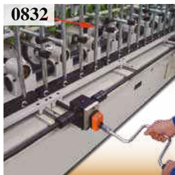
0832 Manual opening of the jamb wrapping tools.
