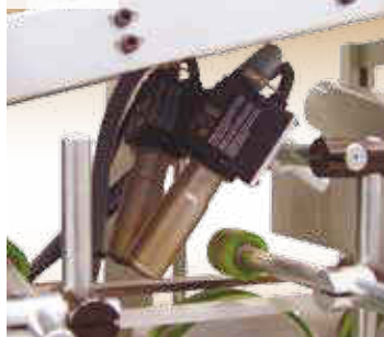
Hot air blower for glue reactivation, PL type.
