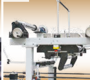
Unwinder assembly with automatic splicing for roll veneer or CPL.
