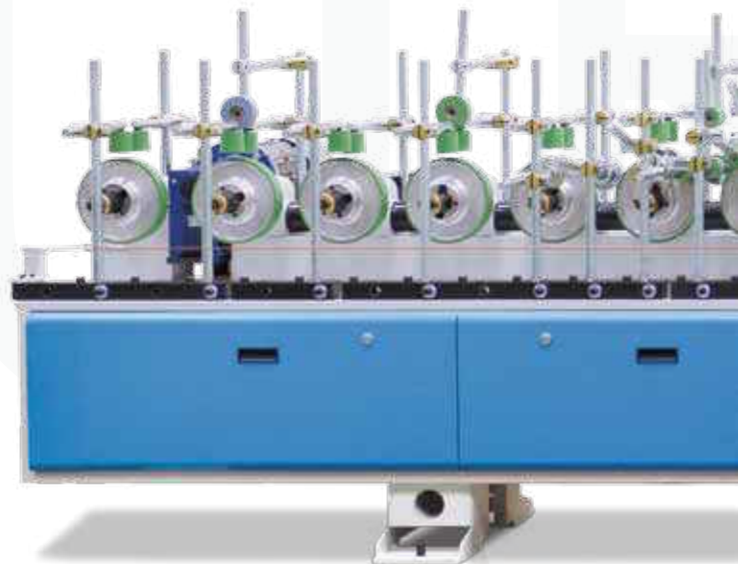
Glue grammage regulation system through PLC. (PUR)
