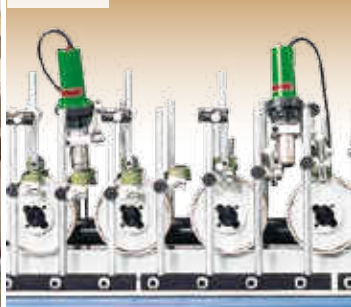
Hot air blower for glue reactivation, RP type.
