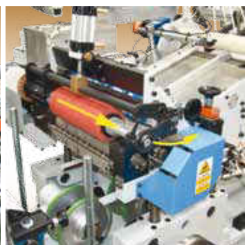
Counter-pressure roller with fast extraction of segments. (PL)
