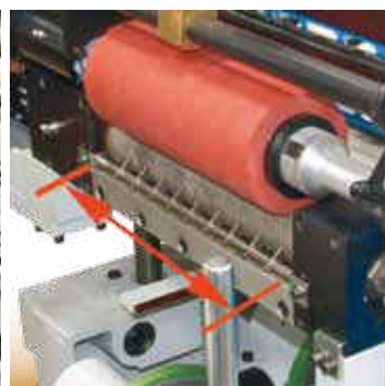
Maximum veneer width 300mm. (PL-32)
