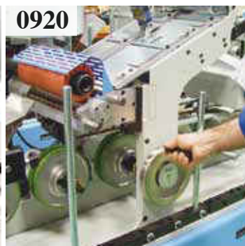
0920 Hot melt coating head lifting system. (RP)
