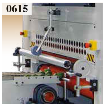
0615 Foil surplus collector at the start of the wrapping process.
