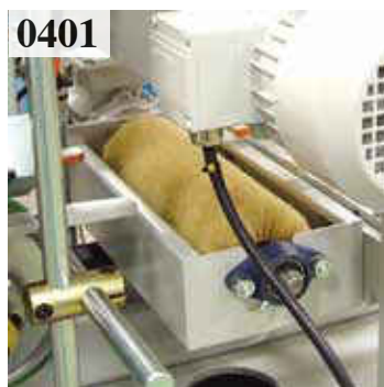
0401 Bottom cleaning brush, to remove the dust from the bottom of the profile.
