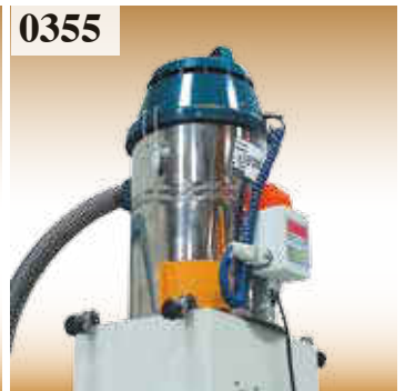
0355 Feeding system for hotmelt granulate to the extruder tank.
