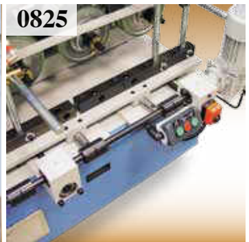
0825 Motorised opening of moulding tools in one side.
