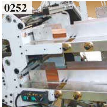
0252 Automatic double feeder of HPL or wood veneer strips.
