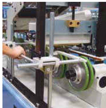
Fast adjustment moulding infeed guides.
