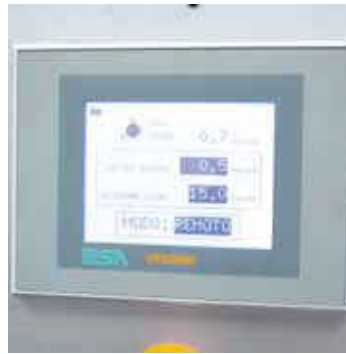
Electronic speed variation 10-60m/min.
