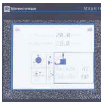
Synchronism timer for the counter pressure roller. (raising or lowering) (RP & PL)
