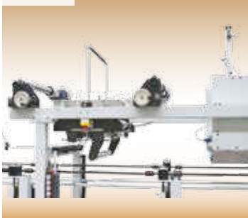
Automatic splicing device for rolled veneer with aluminum strips.
