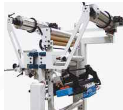
Independent slot nozzle head with double unwinder.
