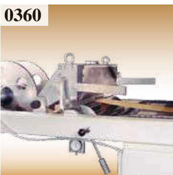
0360 Polyurethane glue application head with eccentric lower roller.
