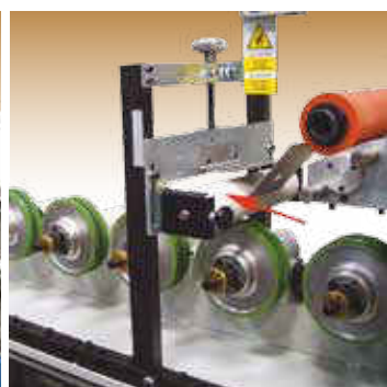
Adjustable first moulding roller. (RP & PL)
