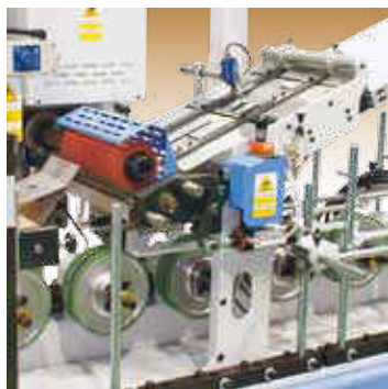
Roller system hot melt coating head. (RP-30)
