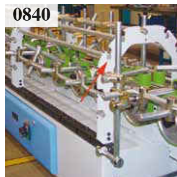
0840 Interchangeable tool-holder cassette/s (2 meter long).
