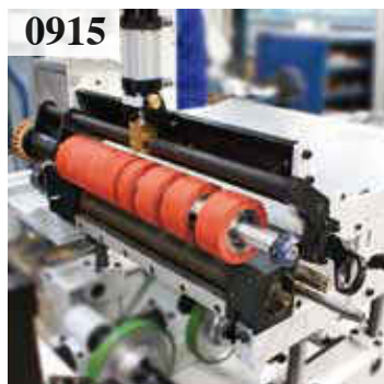
0915 Counter pressure roller fast changing system.
