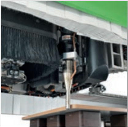
Cold or hot air blower unit to brighten up the colour of the edgbanding strip.
