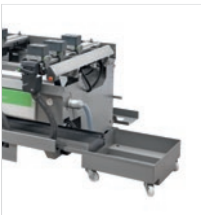
↙ Chip collection basin supplied with the chip mat.
