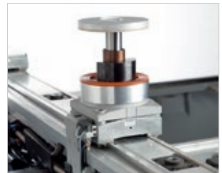
Hyperclamp for rigid and precise locking.
