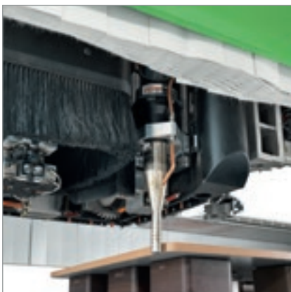
Cold or hot air blower unit to brighten up the colour of the edgebanding strip.
