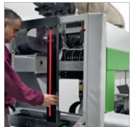
Quick and easy drill change due to the exclusive spindle snap-on coupling system.
