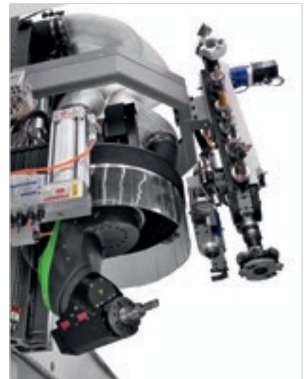
Vertical chain tool magazine on Y axis with 10-15 positions.
