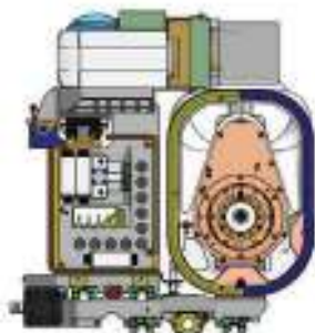
BH 17 Boring Head ( 10 Vertical Drills + 6 Horizontal Drills + 1 Saw blade along X ) + Electrospindle 13.2kW ISO 30 / HSK F63 + 5kW Horizontal Router with ER 32 Collet
