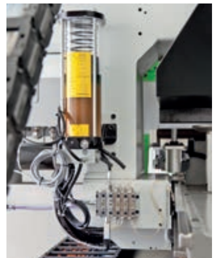
Automatic lubrication is an option that ensures the continuous lubrication of the machine's main moving parts without the need for operator intervention.
