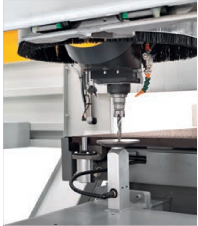
Reduction of tool change set-up time and elimination of operator error, thanks to the contact pre-setter, which automatically determines the length of the tool.
