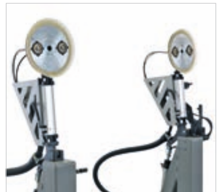
The compressed air-blowing system within the suction pads enables the detachment of thin and porous stacked panels.
