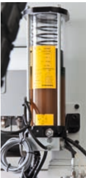
Automated lubrication is an option that ensures the continuous lubrication of the machine's main moving parts without the need for operator intervention.
