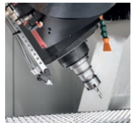
The Air Jet System cools the tool with air at -14°C in order to keep the tool from overheating and prevent the material from melting.
