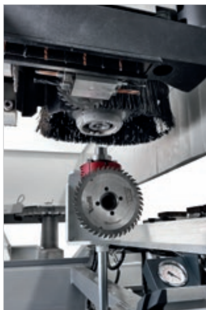
The Pick Up station supports automatic tool-holder rack tooling.
