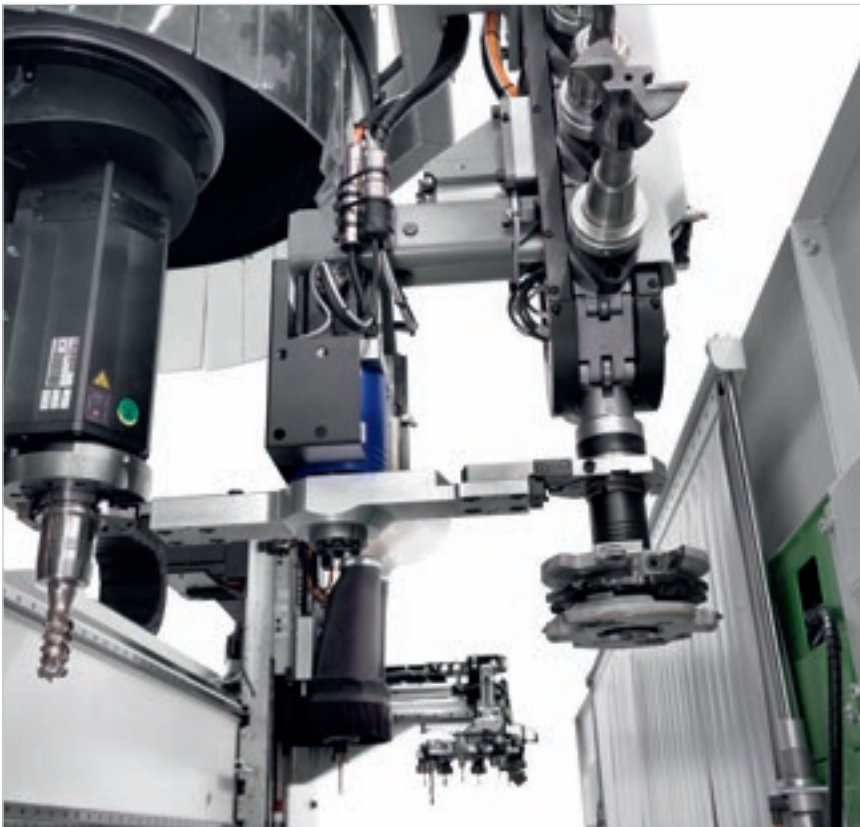
The Pick Up station supports automatic tool-holder rack tooling.
