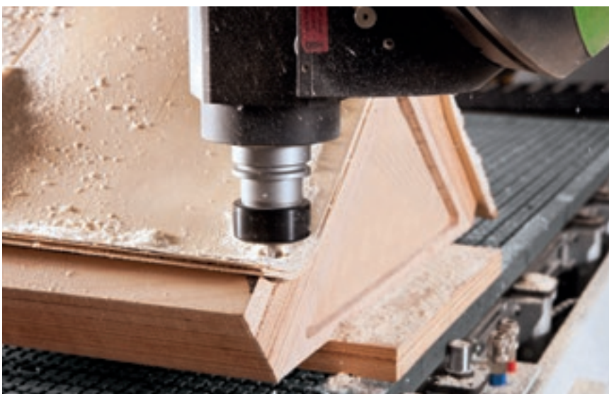
Special vacuum-locking of panels positioned on the jig.
