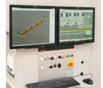
The **CAD/CAM software** used for UNITEAM machines is ideal for designing both straight and curved beams. It was specifically designed for the sector and simplifies machine use, guaranteeing process optimisation and significantly increased productivity.
