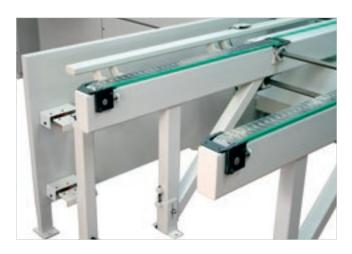
A **buffer**, made up of motorised chains that can collect the pieces, allows for the machine to be fed automatically for a continuous run with no downtime.
