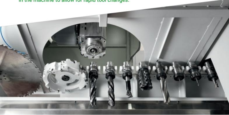
The main milling unit has a tool magazine with 12 positions that can hold a 640 mm diameter blade and a chain-type aggregate.
