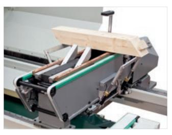
The system that moves the beam through the machine consists of four carriages equipped with vertical and horizontal hydraulic blocking systems.
