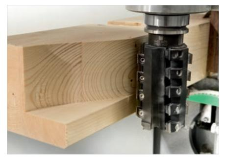
**The 5-axis**, 17kW milling unit, can handle machining operations with large, heavy tools thanks to the encoder placed on the spindle axis, which regulates the current used, based on the advancement of the tool.
