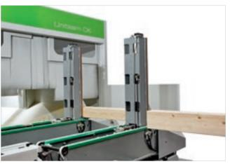
The clamps have a **90° hydraulic rotation system** that allows for all six faces of the piece to be machined without needing a second intervention.
