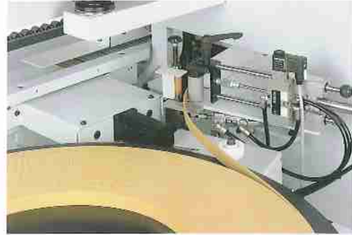
Automatic infeed device for coil material from outside of the hood area (optional).
