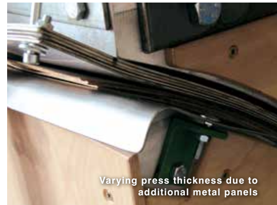
Moulding the heating plate
