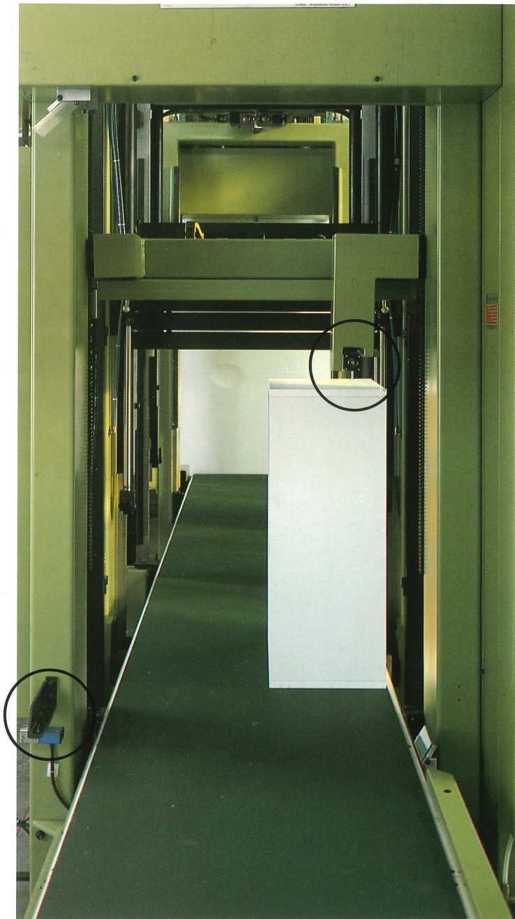
Sensor to read the cabinets length and height; conveying and clamping in asymmetric cross position.
