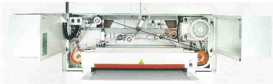
The "TAC" combines the sanding power of the crossbelt unit with the fine control of the "EPICS" sectional pad. This ensures excellent results even on the most difficult jobs, such as removing glue or joint paper from veneered panels or superfinishing painted panels.
