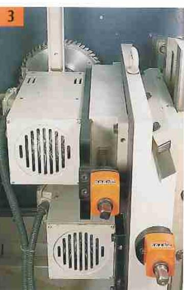
**3. Double hogging**, with slide support (patented), equipped for vertical and horizontal movement (both may optionally be automated). It is made up of two pulversifers which are superimposed in the central area, and which are set automatically when the height of the piece is changed. Optionally, horizontal and vertical movements may be automated.
