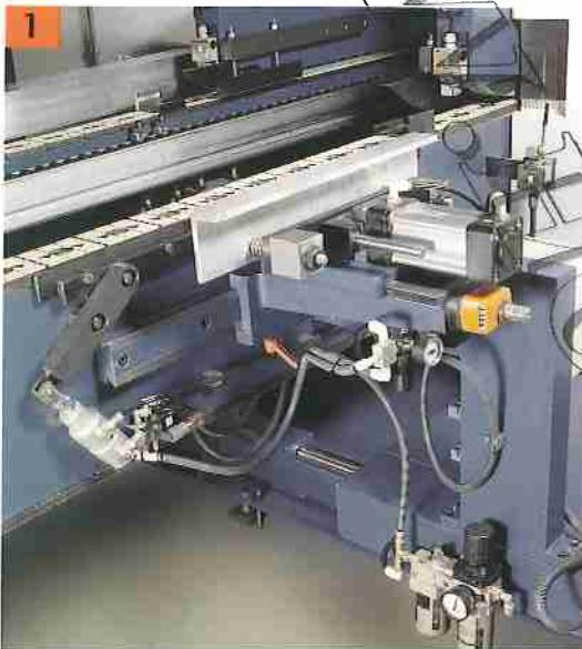
**1. Height stop device and centring devices**, for auxiliary machines performing the square-cutting operation. This holds the panel until the stops make contact with it and reference it.
