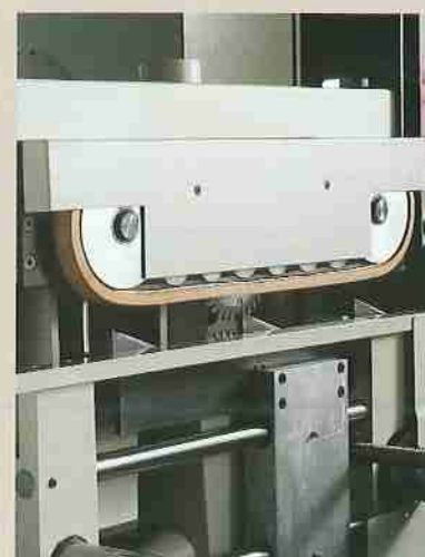
HOLD-DOWN system with heavy-duty rubber belts to increase work-piece stability while trimming and prevent face marking
