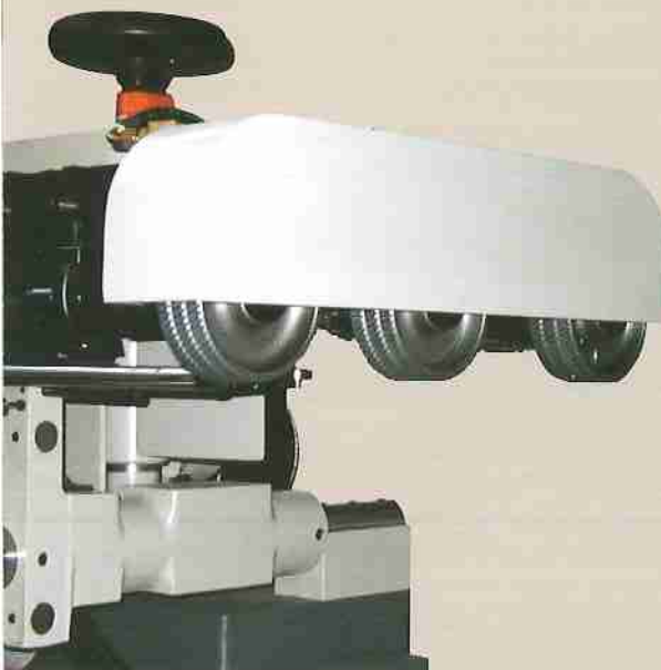
THIRD DRIVEN FEED ROLLER to improve loading consistency of short pieces and increase feed power for generous cross sections
