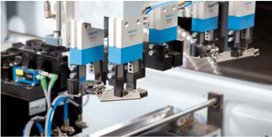
Pick&place feeding system, e.g. for plug hinges
