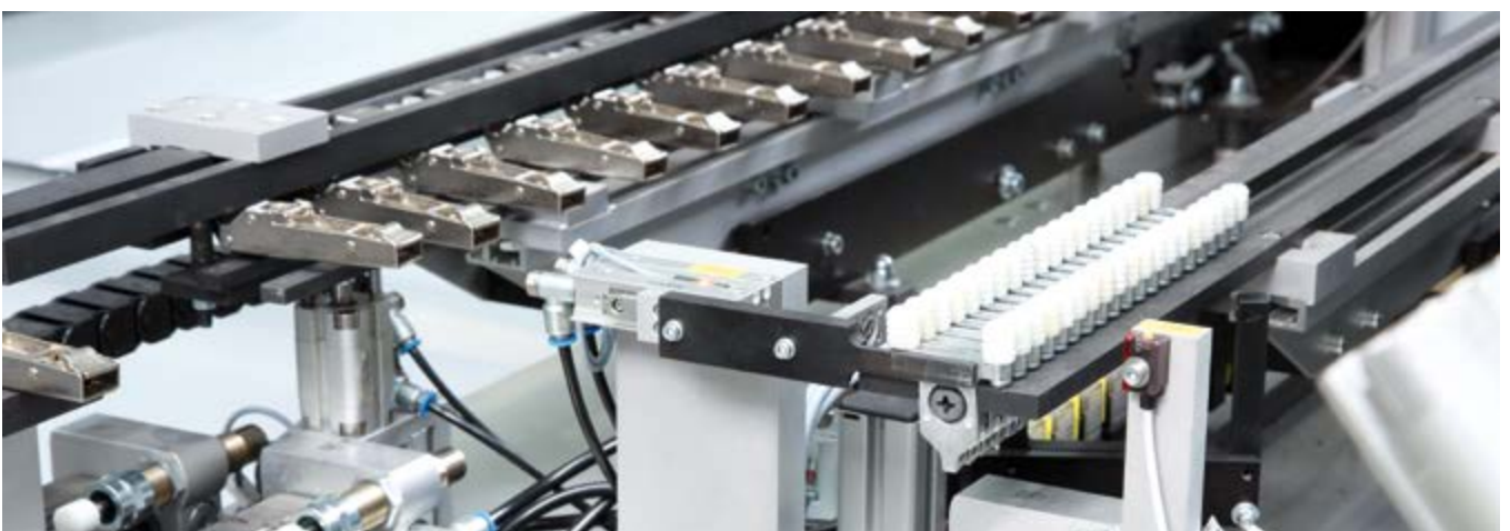
Linear transport section to transfer and separate hinges
