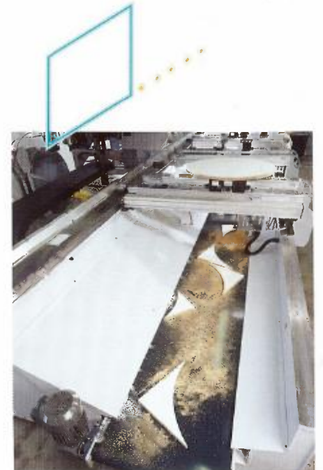
Disposal of residue pieces with chip conveyer belt
