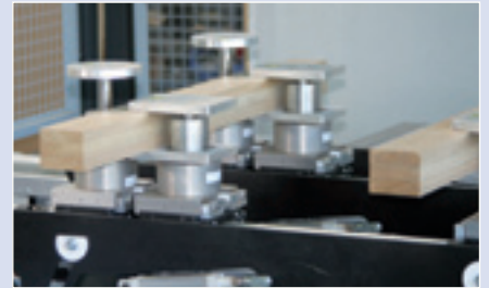
Automatic reclamping for 5-sided processing of window and front door staves.
