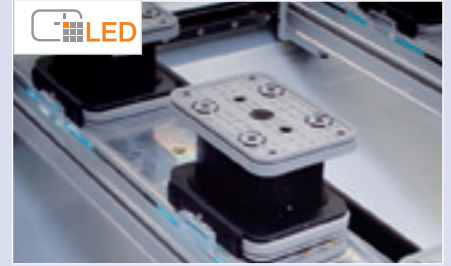
LED system – both the fastest and safest positioning system for consoles and clamping elements (patented).
