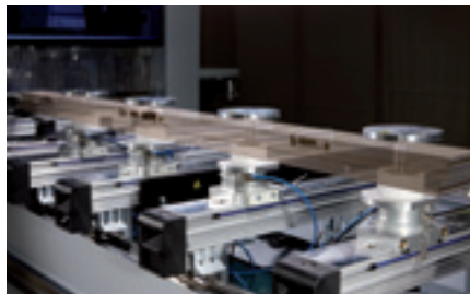
Manual clamping fixture powerClamp for straight and curved parts. Ideal for all arched, narrow and frame parts.
