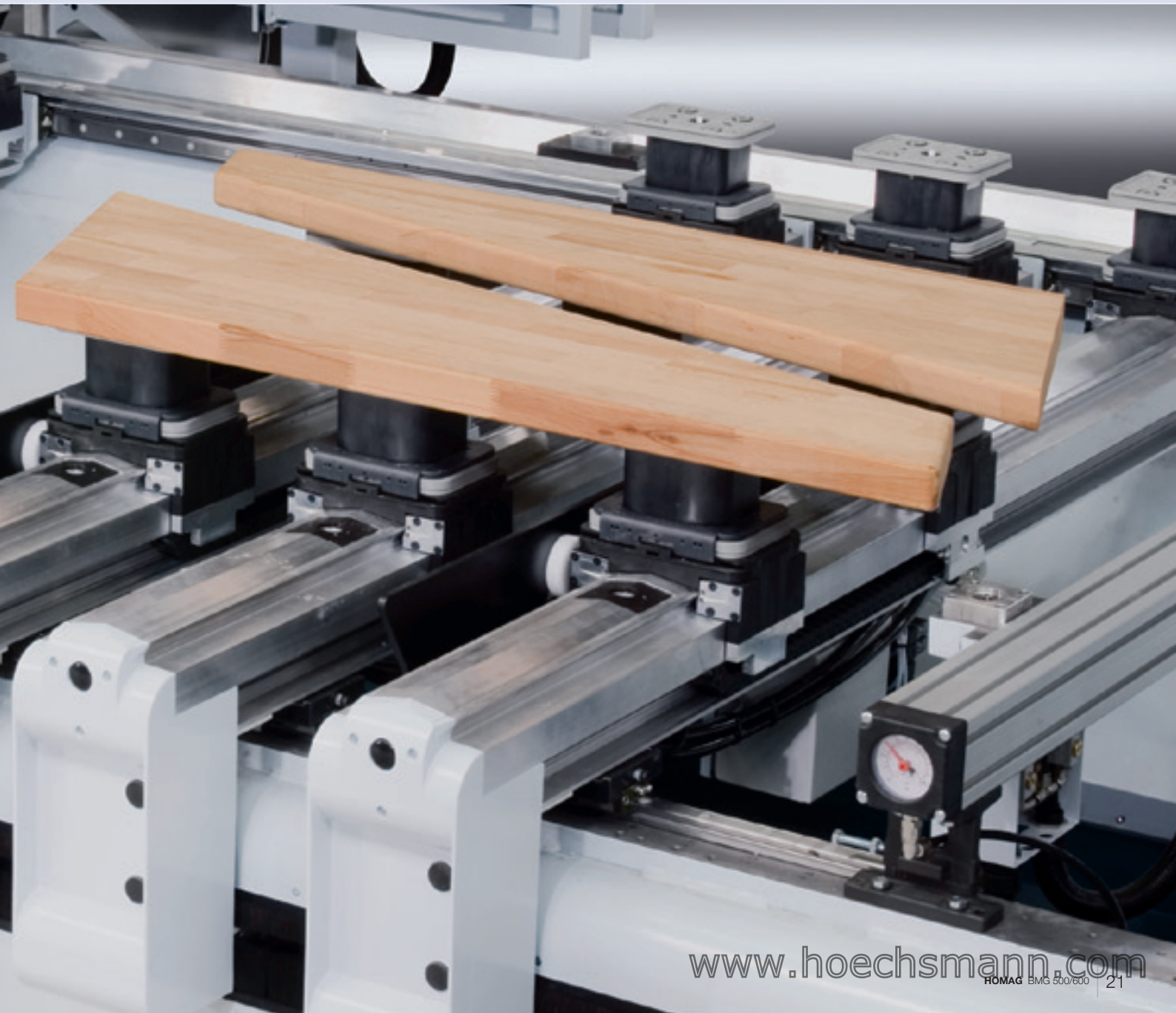
Automatic cutting and separation of staircase treads for all-round complete processing.
