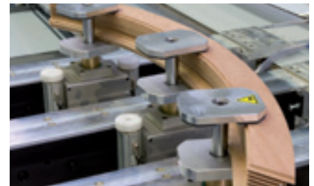
Highly rigid 3-step clamps with extreme clamping height for precise complete processing of window and front door components without subsequent outside moulding and profiling.
