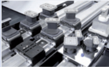
Different vacuum and pneumatic clamping elements guarantee precise processing of different workpieces and materials.
