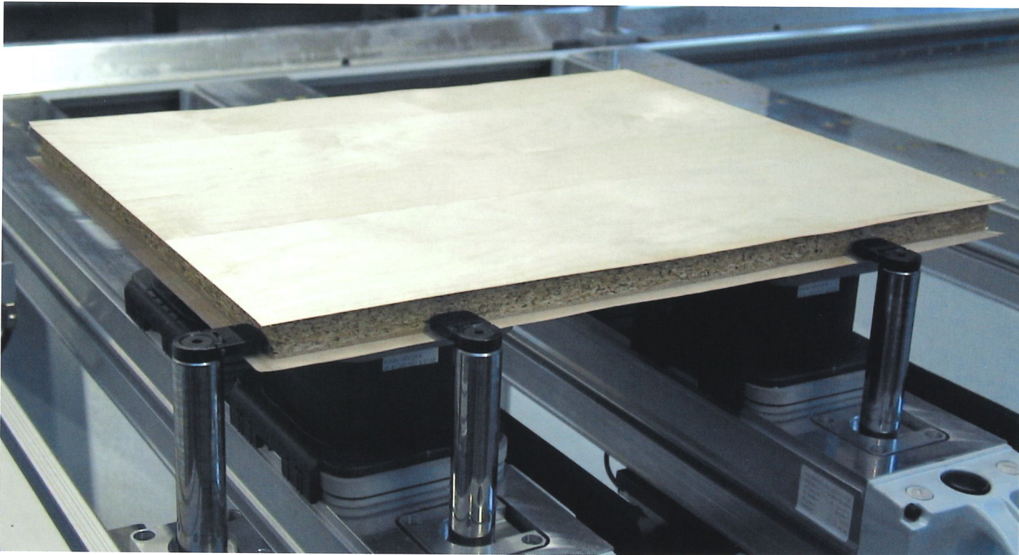
Locating pins with removable sleeves for workpieces with overhanging laminates (such as veneers). Alternatively, rotating pop-up locating pins with tabs for overhanging laminates are also available.
