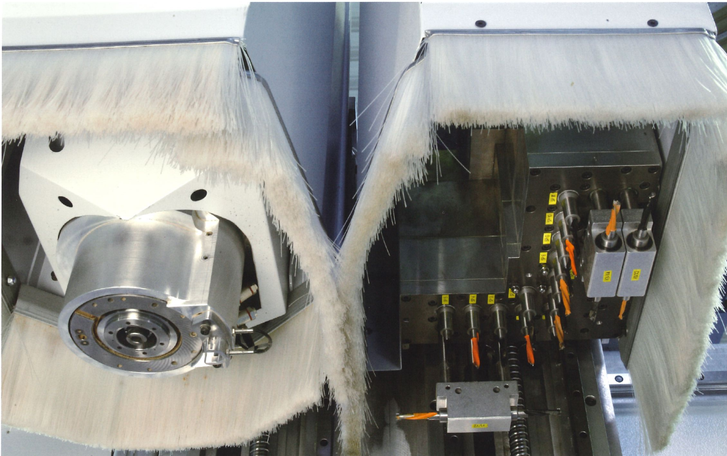
Working spindle and drilling head with separate Z axes for tool changes on the working spindle during application of the drilling head (Option Performance Pack).
