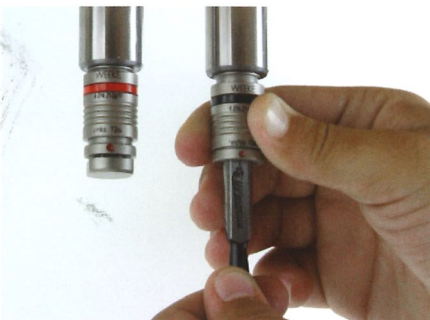
The patented high-speed drilling head change-over system permits the drills to be exchanged without the need for tools.
