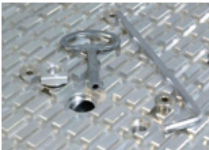
1" vacuum connections with quick-open function by means of switch cabinet key, vacuum openings with precision thread for fixing clamps
