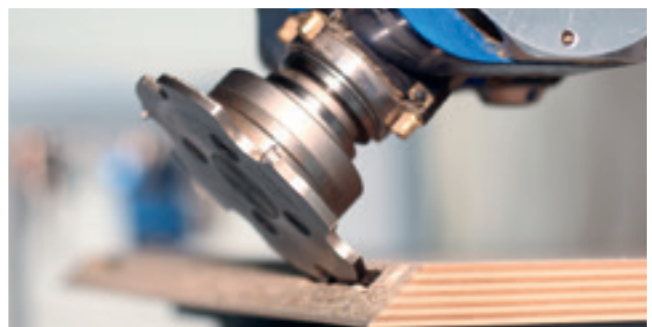
Cutting recesses for connecting fittings
