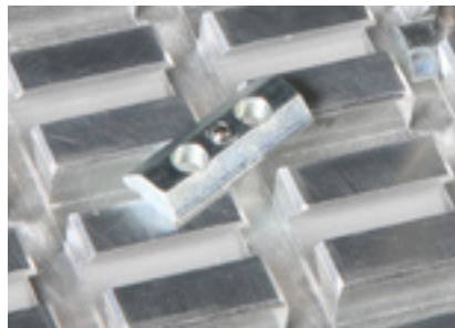
Slot nuts with thread for positive locking of clamping fixtures in the dovetail guide.
