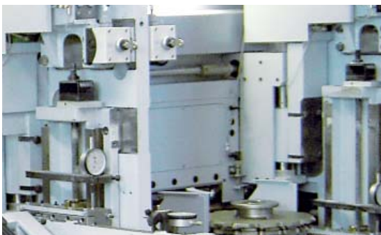
Horizontally adjustable top pressure with digital position display
