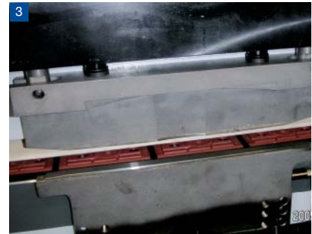
Pressure and support pad (for laminate) to protect the chain and ensure precision processing. With DBS, the workpiece is traversed in a guide fence
