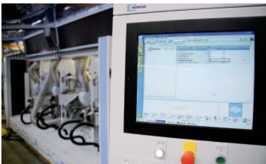
Easy-to-operate powerControl system in accordance with IEC 61131, with facility for remote servicing and diagnosis
