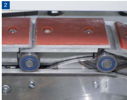
Rolling chain (DBS belt in the powerLine or magnetic chain for high outputs)
