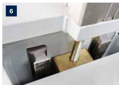
6 Linear guide for precise adjustment of the top spindles for optimal work piece quality
