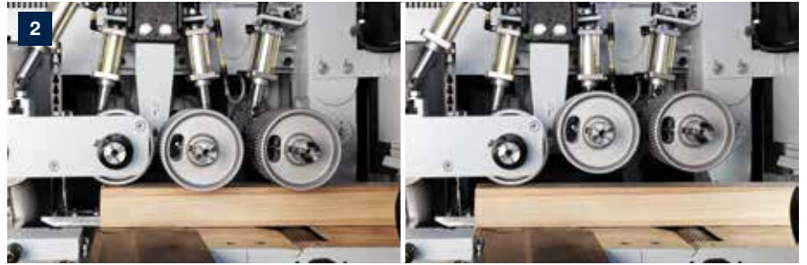
2 Pneumatic adjustable top feed rollers for optimum contact pressure for different profiles and types of wood (left activated, right deactivated feed rollers).
