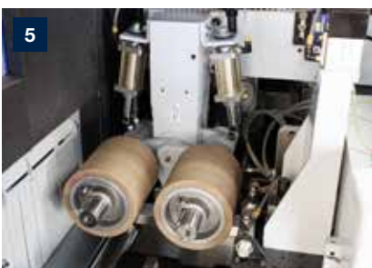
5 Top pressure rubber rollers for sensitive surfaces after processing (Shore hardness: 80)
