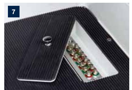
7 Accessible central lubrication at machine front
