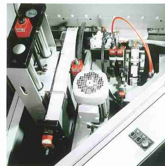
Central cutting flange For separation in the range from 140 to 310 mm, providing twice the output when processing double widths.
