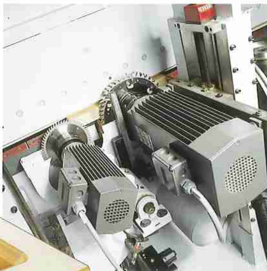
Scoring / hogging Perfect sizing without tear-out, also for coated substrates. Pre-scoring unit with lift-out device. Hogging unit with cross support and extractor hood.
