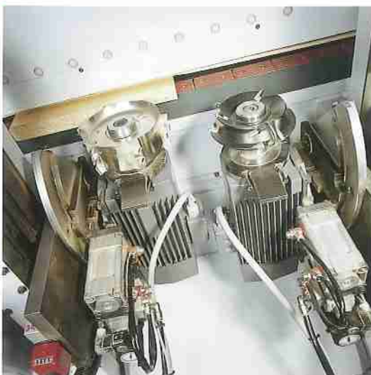
Standard trimming unit For finish trimming, rebating, profiling, grooving etc. Electropneumatically controllable, swivel range 90°. Cross support and reversing switch to govern the sense of tool rotation.
