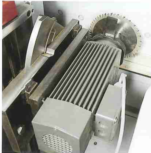
Prescoring saw above For splinter-free processing of coated surfaces or for clean-cut transverse processing of veneered parts or solid wood. Scoring motor 2.2 kW Tool diameter max. 180 mm
