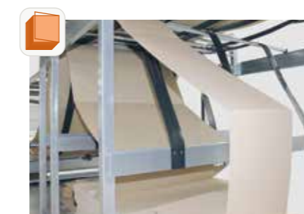
The endless cardboard change system is an automatic change system for endless web, from six compartments of various widths.
