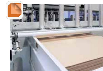
The automatic single sheet feeder with lift table allows the automatic feeding of stacked single sheets.
