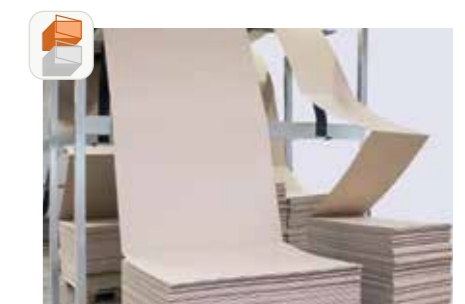
In the Side by Side operating mode, the cardboard feeding compartment is expanded by one more web width, allowing single sheet access to up to twelve web widths in a sixcompartment change system.
