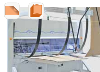
The combination cardboard feeder allows the automatic feeding of single sheets or using endless cardboard.
