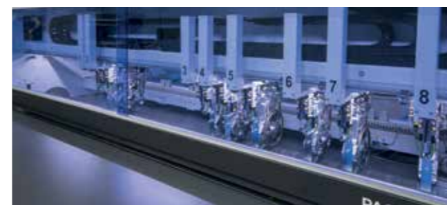
By means of fully automatically movable and quickly repositioning cutting tools , almost any blank can be produced.
