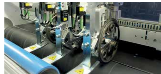
Tools running on rubber rollers provide for lower cutting force and lower wear-and-tear, at best cutting quality and long tool life.
