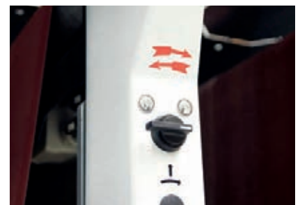
Optional Cutting direction ▪ Cutting direction either with or against the feed direction. Different cut directions ensure maximum fiber reduction. Particularly important when combined with water-based paint systems.
