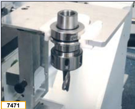
7471 Tool transfer station, reliable, fast loading of the tool changer including empty slot interrogation in the tool changer
