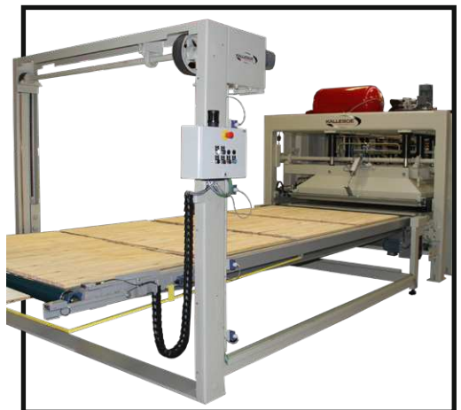
Board stacker for automatic stacking of finished boards
