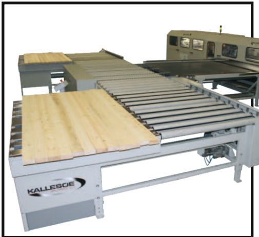
Sorting equipment KS1 double sorting equipment for manual sorting
