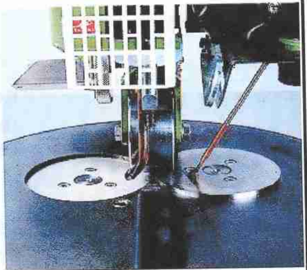
Specific feature of all KUPER splicers: the discs with tolerance-compensating mechanism. Thickness tolerances of the material are compensated.
