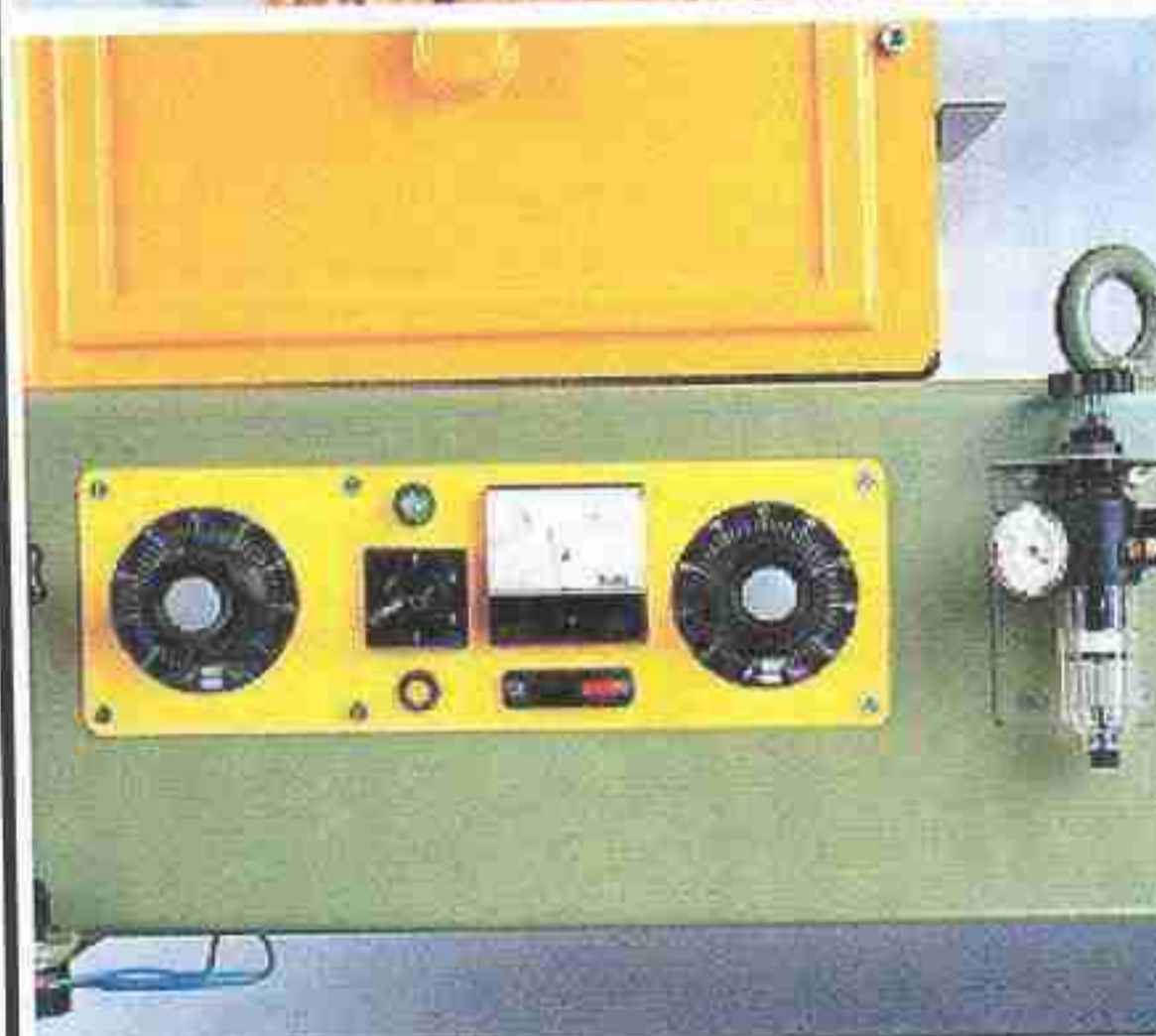
Control panel with ammeter and two transformer regulators for separate regulation of the heating power in standstill- and running-mode.
