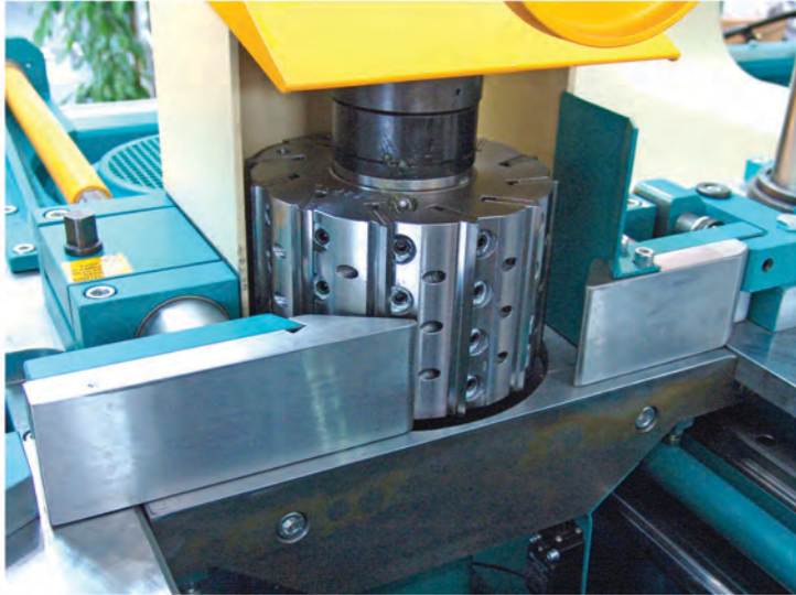
Vertical spindles can also be adapted for moulding.
