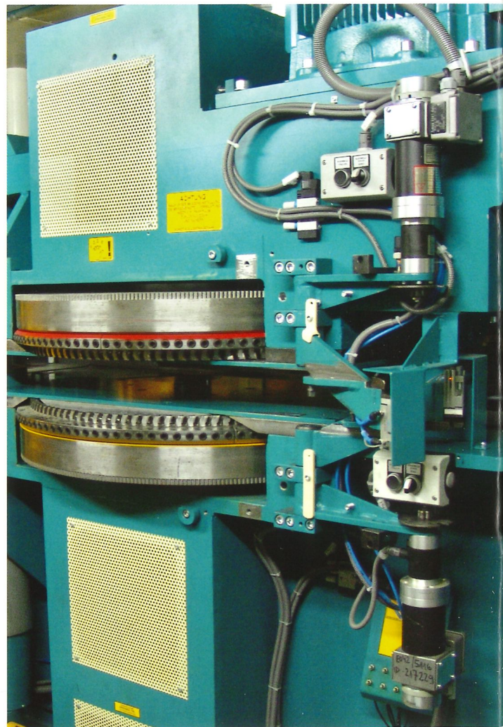
High precision of horizontal planing is achieved by a very short distance between the two rotors.
