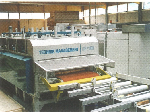
Hochfrequenzpresse für BSH. High-frequency press for laminated beams.
