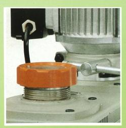
High-low variable speed unit with expanding pulley.
