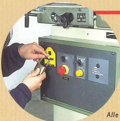
All CE-mark machines are fitted with a padlocked main switch, overload protection, emergency stop pushbuttons in the working area and safety limit switches to prevent damage to the machine or injury to the operator.
