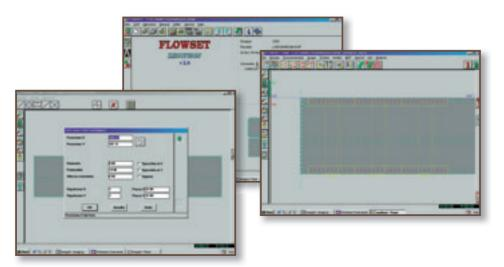
FLOW-SET uses the CAD drawing to draw the drilling diagram and to automatically configure the position of the units and the heads. The program can also check the feasibility of the drilling diagram, warning of any incompatibility with the machine configuration. In the P.C. version of Zenith, the positions are transferred to the machine via a serial port or with a disc.
