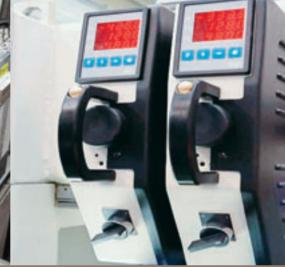
The pressers, thanks to a pneumatic system operated with a pushbutton located in easily accessible positions, raise and position themselves in the upper part of the beam, leaving the machine completely open for the various fixturing operations.
