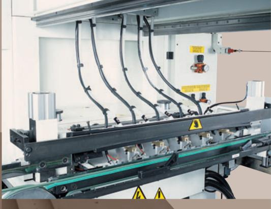
In the dowel gluing version, the machine is fitted with horizontal dowel inserters. They are constantly supplied, through a special circuit, from two containers with vibrators to ensure that the dowels do not iam.
