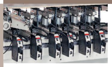
Switching from one program to the next, the control unit sends to all the displays the differential quotas between the old and the new program: the operator must simply move each unit in the direction indicated on the display until the value is zeroed.
