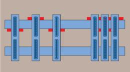
The dimensions and structure of the pads ensure that the groups are perfectly balanced . The supports, in fact, by sliding alternatively on the two THK guides fitted on the sides of the beam, penetrate each other, allowing the units to be brought together by up to 96 mm.
