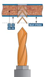
Higher quality drilling in faster times. The machining heads are fitted with coaxial motors at the spindles and an inverter that manages the power generated by the motors to achieve a uniform rotation speed in any situation.
