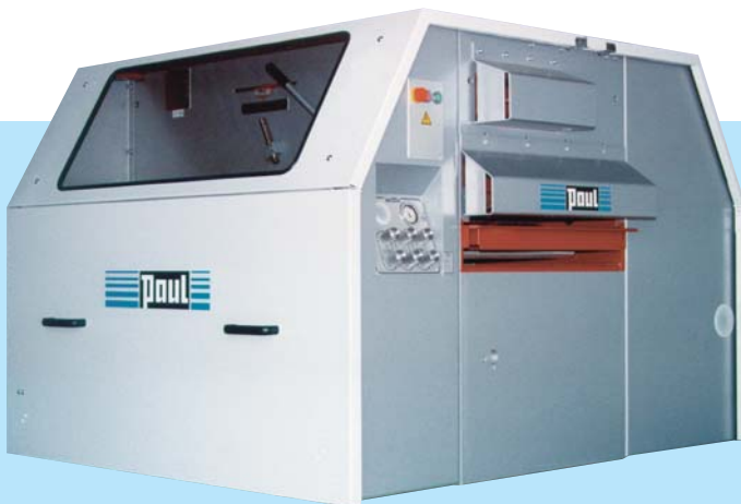
Fig. 8 Model K34G/800 (opening width 800 mm)
