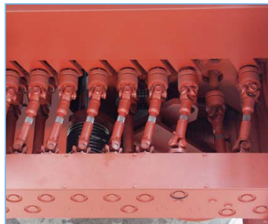
Fig. 20 Drive of feed rollers via cardan shafts
