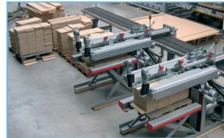
Fig. 37 Length-sorted stacking of cross-cut workpieces on pallets
