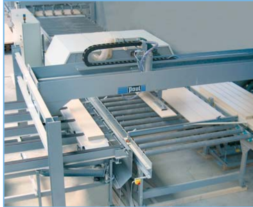
Fig. 35 Vacuum gantry stacker for stacking the strips leaving a K34G/2200 multirip saw with automatic infeed system
