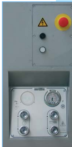
Fig. 11 Operating panel of a K34G
