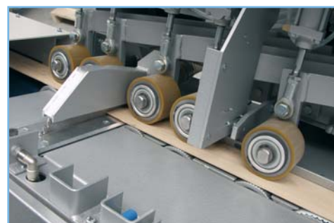
Fig. 42 ... an automatically linked CNC cross-cut system
