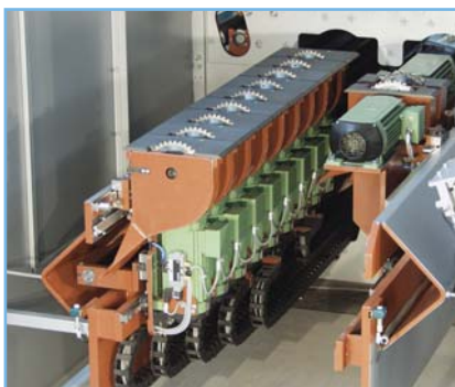
Fig. 34 Lowerable saw heads
