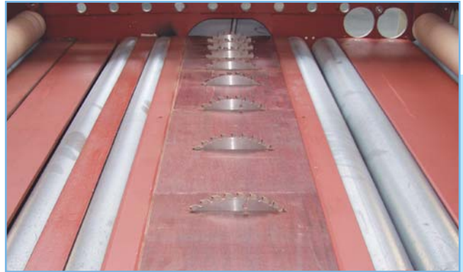
Fig. 10 Insert table with rip saws and bot- tom feed rollers
