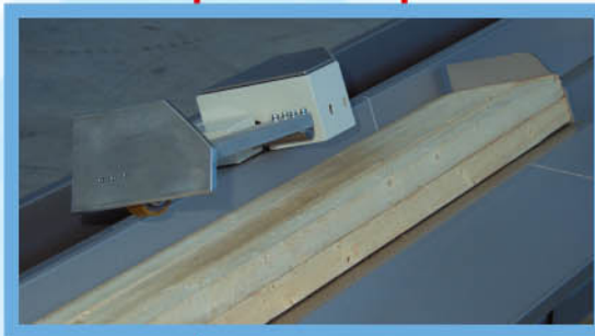
Fig. 16: The output is increased significantly when cutting several pieces packed together.
