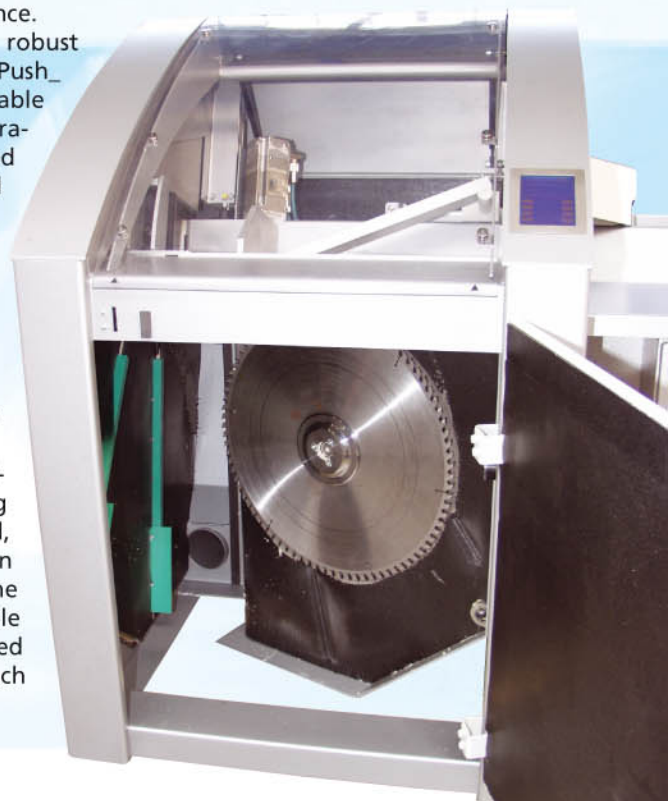
Fig. 3: Convenient saw blade replacement from the front
