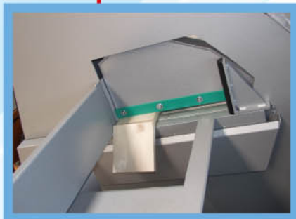
Fig. 10: ... automatic disposal of waste offcuts up to 250 mm long
