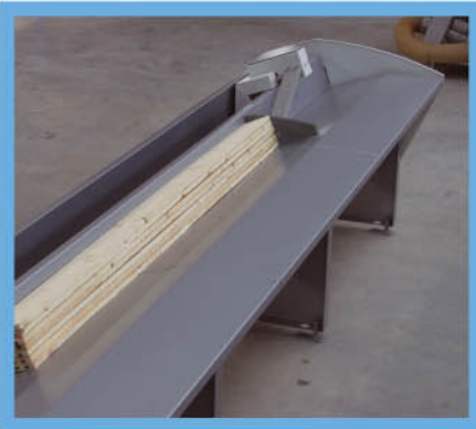
Fig. 4 + 5: Upward tilting standard pusher enables length measurement & crayon mark recognition – also ideal for cutting timber packs.
