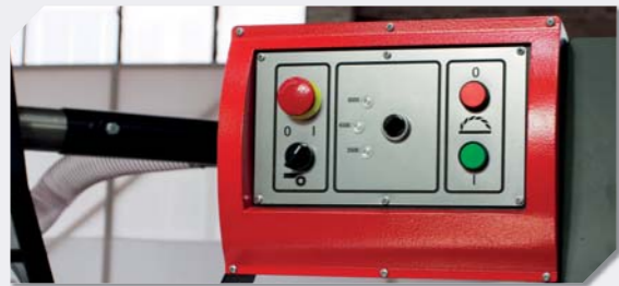
Spindle rotation speed set adjusted from control desk.
