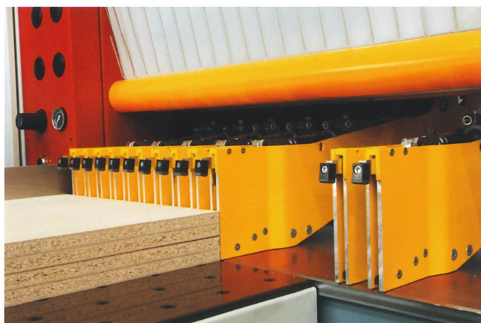
Push off and push out with the grip-push clamps ERGONOMICS PLUS+
