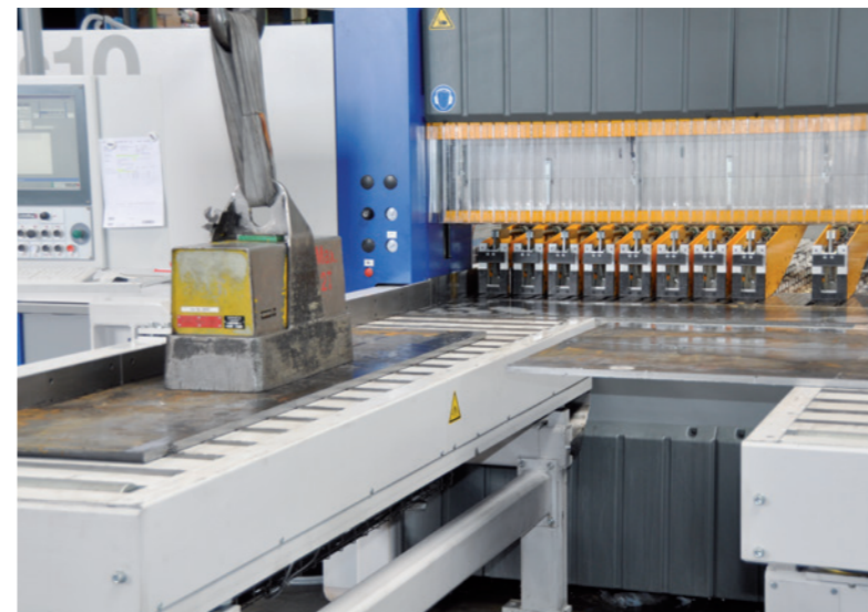
... which are placed on the roller table at the angle stop.
