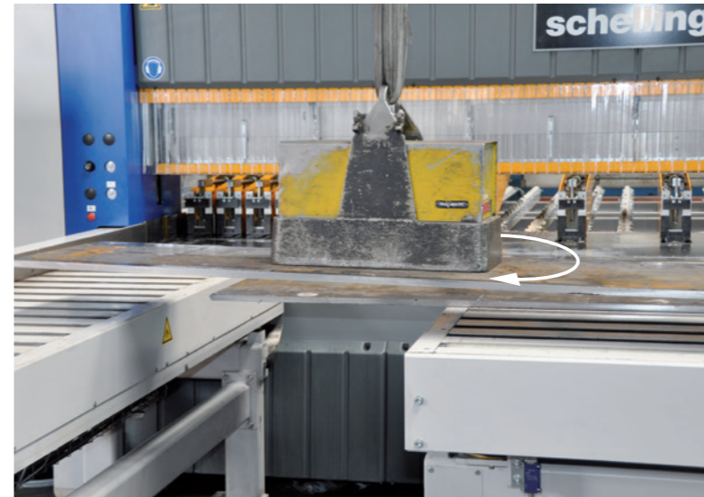
The crane is used to turn the strips by 90 degrees ...
