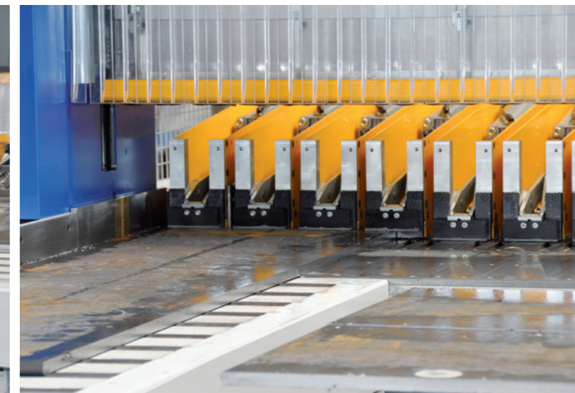
By pressing the start button, the strips are clamped and cut up.
