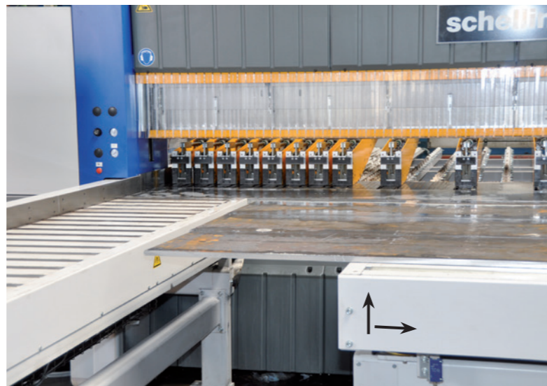
The roller table is lifted and pushed to the right with the material.
