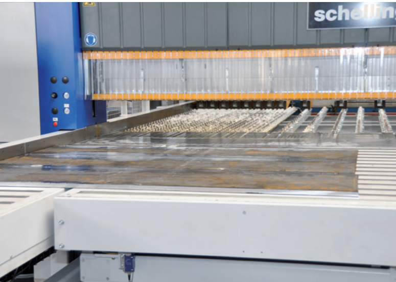
The scissor clamps push the sawn strips out of the machine completely.
