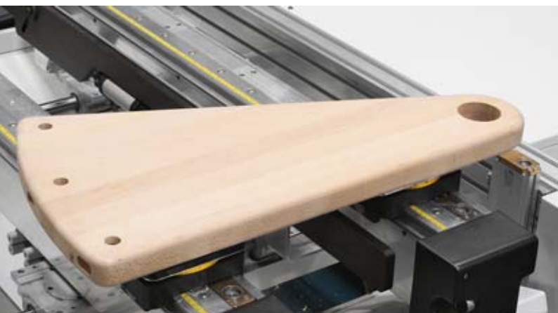
Vacuum cups to hold down pieces of any shape, from the element of solid wood or panel door to those of scale.
