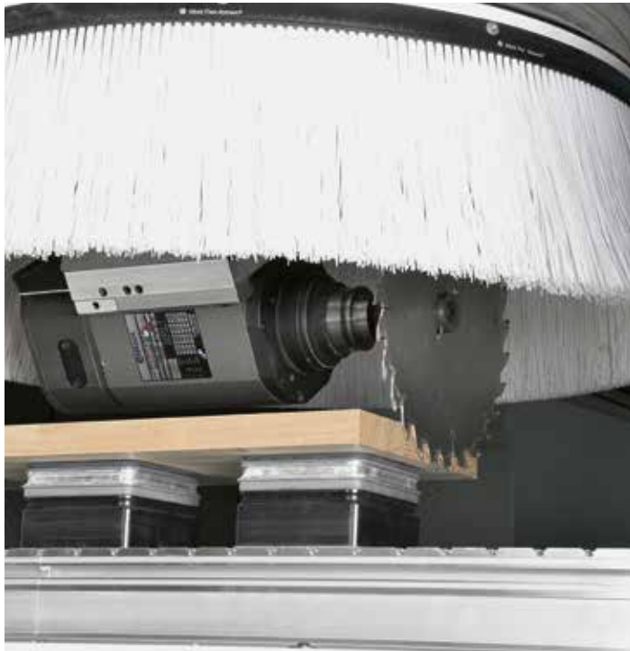
The outer hood is used during 5 axes routing operations, as it has adequate dimensions to cover all tool movements.
