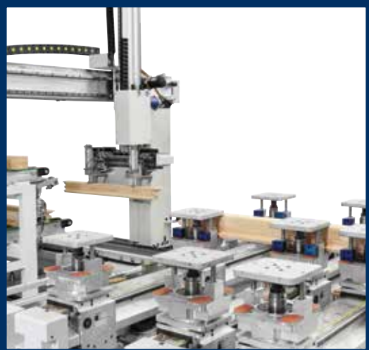
Flexible work cell for the production of window and door frames, fitted with automatic loading and unloading.
