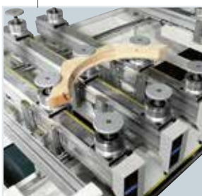
Bars worktable configurable with clamps and suction cups, ideal for the processing of solid wood.
