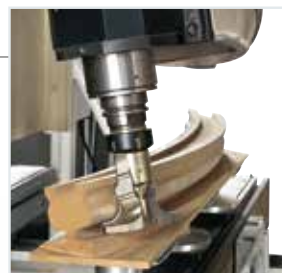
PRISMA machining head with 5 axes electrospindle.
