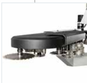
Chain tool store with 32 positions anchored to the mobile gantry structure, developed for managing heavy and large tools.
