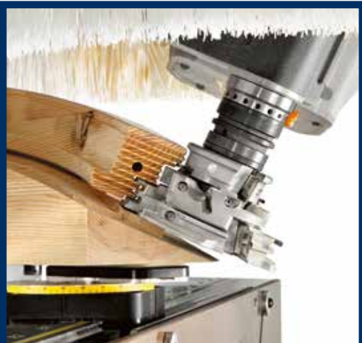
PRISMA machining head with 5 axes electrospindle.
