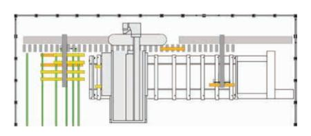
The cycle is completed by unloading the elements from the right half-table, while the machine is already machining the next elements on the left half-table.
