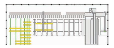
The left handling unit picks up the unfinished workpieces from the loading buffer (upper table) and deposits them on the left half-table.
