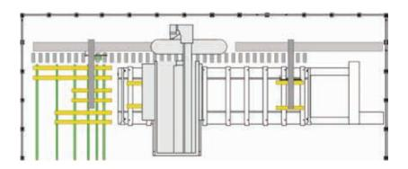
While the machine executes the program on the left half-table, the right handling unit receives the next unfinished elements from the rear roller conveyor and deposits them on the right half-table.
