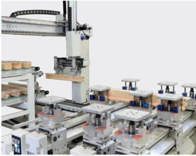
The handling units are positioned with NC controlled axes. The clamping devices are positioned automatically, according to the length and width of the work-pieces.
