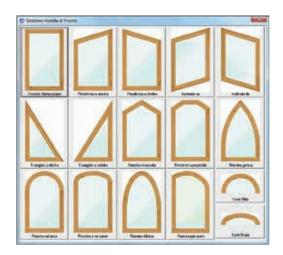
**Parametric software** developed by SCM to design and produce door and window frames on work centres. Supports the design requirements of the most common types and geometric shapes of door and window frames, both linear and curved.
