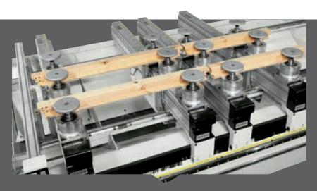
Matic is the fully automatic worktable ideal for machining solid wood. Complete set-up in seconds, all bars and supports moving simultaneously, each driven by an independent motor. The many technical devices give this table lasting safety and reliability.
