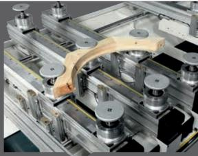
Perfect for machining pre-finished/ finished door and window frames, all supports having cleaning blowers which remove all shavings from the sliding zone and on the workpiece hold-down base during clamp changes.
