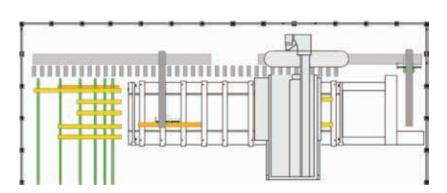
Once the program is finished, the left handling unit unloads all the finished elements from the left half-table and deposits them on the unloading buffer (lower table).
