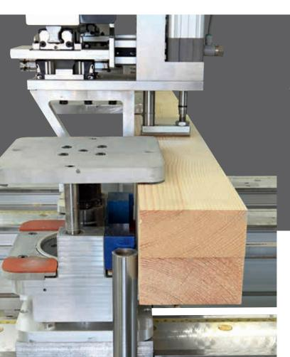
The square shaped hold down clamps are designed to efficiently block linear workpieces of any section; they are indispensable to hold down short workpieces.
