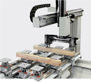
Several elements, of different length, can be positioned on the loading buffer. When the operator loads the element, its dimensions (length, width, thickness) are checked with an optical sensor.
