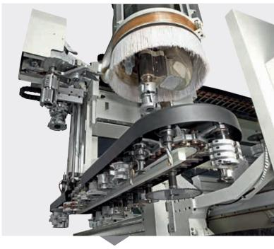
The machine is always equipped for any machining using the TRC chain magazine with 48 locations available for large and double-profile tools.
