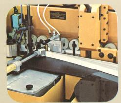
The automatic B3 and B4 edge banders have been designed to rationally resolve all edge banding problems out of machining line.
