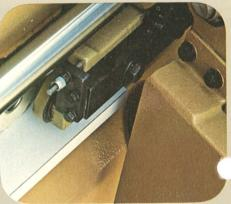
In this way, the B4 produces accurately chamfered corners using only one end cutting unit instead of the traditional two, occupying less space and enabling a reduction in consumption of electric current and servicing time.
