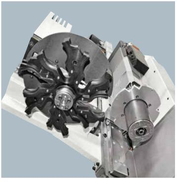
**AUTOMATIC TOOL CHANGE: RAPID 6**6-position tool store for maximum tool diameter up to 150 mm. Plastic collets for tool locking. Fast rotation by brushless axis.
