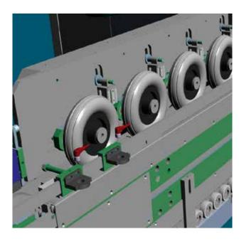
Device for automatic feeding of panels from handling equipment to machine infeed.
