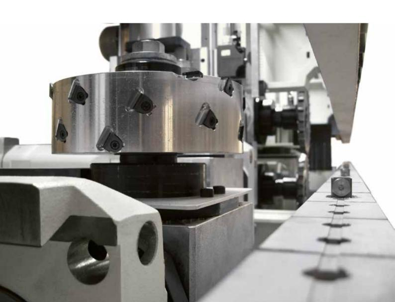
Top pressure beams with spaced pulleys and vertical adjustment according to work piece density, dimensions and profile to always guarantee a precise and uniform movement.
