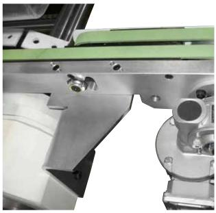
Double belts at machine infeed and/or outfeed with speed regulated by inverter.
