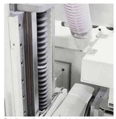
Protective accordion devices against abrasive dust prolong the life of mechanical parts and significantly reduce maintenance.
