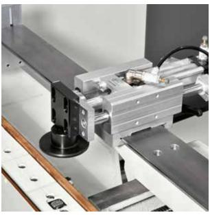
Aligning device to center the panel perfectly.
