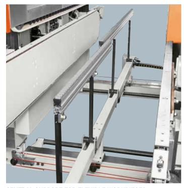
**CENTRAL SUPPORT FOR FLEXIBLE WORKPIECES.** It can be a plain shaft support or with rollers; manually adjustable, fixed or retractable self-centering.
