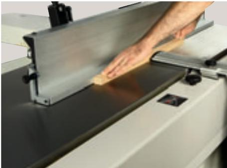
The **additional overturning fence**, integrated in the surface fence, ensures a perfect operator's safety when machining small workpieces. Available on request
