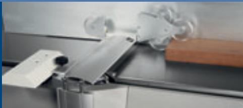
Roller with two different types of rubber to simultaneously process several pieces with different thickness.
