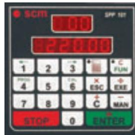
Electronic positioner of thicknessing table.
