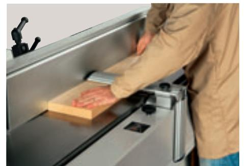
The **cutter block guard is incorporated in the machine base** (patented device). This is just another example of SCM's commitment to providing the woodworker with the best and safest working conditions. Included in the standard equipment
