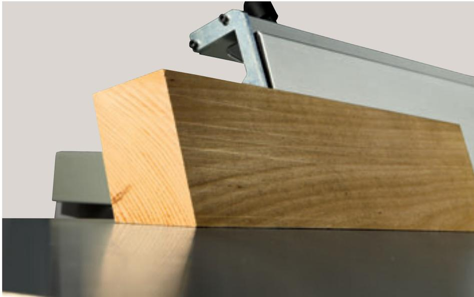
The **rectified worktables** ensure the best quality when machining, a very low roughness and a perfect planarity.
