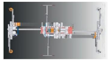
The suction cups support table adapts automatically to the dimensions of the boards.
