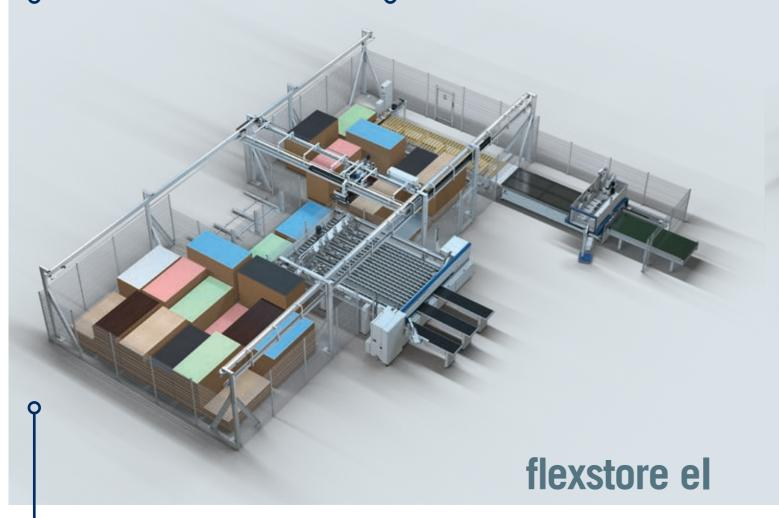
**Increased quality** thanks to the accurate and precise handling of the boards with the pickup table fitted with systems designed specifically to maintain the surface finish.
