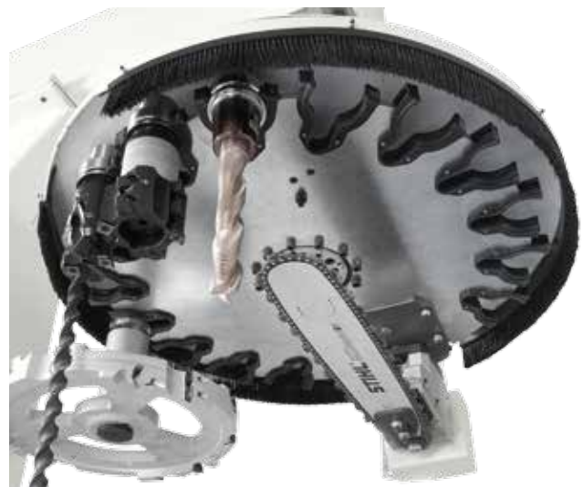
Dedicated position for chainsaw or tools of weight up to 15 kg
