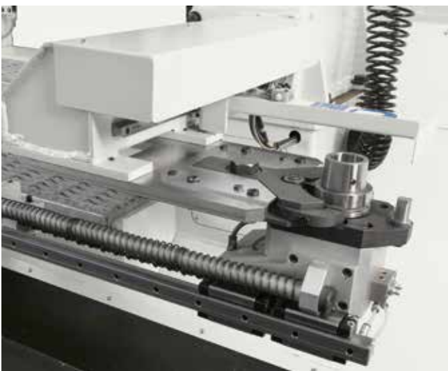
Dedicated position for mortise chain or tools of weight up to 15 kg
